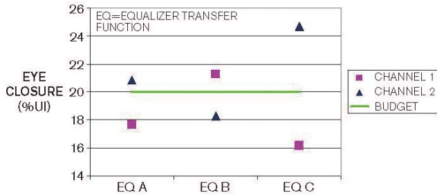
Figure 6 You can use equalizer transfer functions to equalize two channels of an 8m AWG32 cable. EQ A is a reasonable but not optimal choice for Channel 2, EQ C is the best transfer function for Channel 1, and EQ B is the best transfer function for Channel 2.
